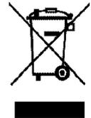
The symbol on the product, or on the documents accompanying the product, the Crossed Out Wheeled Bin, indicates that this appliance may not be treated as household waste. Instead it shall be handed over to the applicable collection point for the recycling of electrical and electronic equipment, or, if you are buying an equivalent product, to the retailer of the new product.
