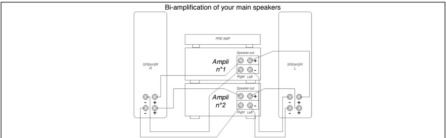
Instead of two amplifiers, you can use a single amplifier if it is equipped with two sets of speakers A and B. Both sets should be selected. This is biwiring and not bi-amplification.
