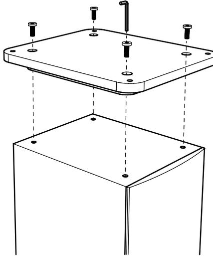
2- Screw the pedestal using the supplied key
