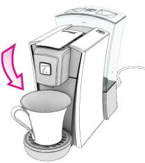
Press until water tank is empty and discard the water.
