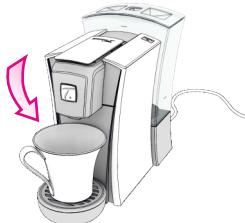
Press until water tank is empty and discard the descaling agent.
