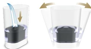
Install new water filter. Fill water tank half way with fresh drinking water. Then tilt the water tank back and forth to remove air bubbles from the water filter.
