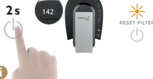
Press power button for 2 seconds to display the remaining cups brewable with the water filter (max. 150). Note: Water filter must be changed when RESET FILTER indicator lights up orange.
