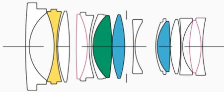
■ SLD glass ■ FLD glass ■ ELD glass ■ ASPHERICAL LENS
