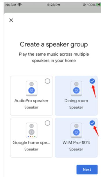
Since the WiiM Pro is a Chromecast audio receiver, not a transmitter, it can't transmit the Line-in or Optical-in audio to other Chromecast audio devices such as Google Home.
