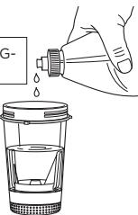
Fill with warm water up to top of Power Paddle and add 1 or 2 small drops washing-up liquid. Install blade assembly.
