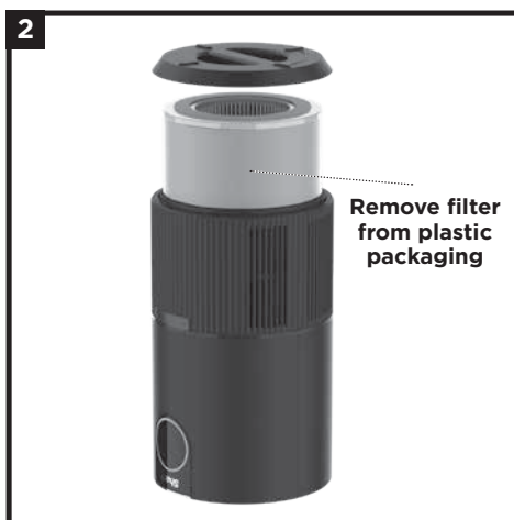
2. Take the filter out of the unit and remove packaging, then insert back into the unit. DO NOT run the air purifier unless the filter is removed from its packaging and properly reinstalled.
