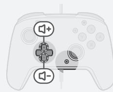
**EN** A. To adjust the controller's volume, hold down the "function" button and press the Up/Down on the D-pad.
