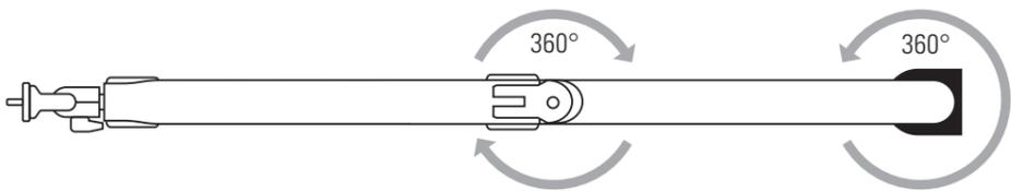
Flexible mic positioning with rotatable ball-head.
