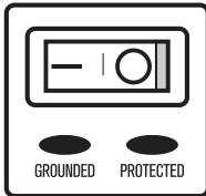
The green "ground" light should turn on when power is supplied by your Monster Brand Surge Suppressor. This light indicates that your unit is properly grounded. If this light does not turn on, it is an indication that your unit is not properly grounded and you should contact a qualified electrician to properly ground the outlet. Use of a Monster Brand Surge Suppressor that is not properly grounded will void all terms of the Connected Equipment Warranty.
