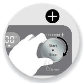
2- Next, adjust the parameter(s) using the +/- selector (C14). For safety reasons, it is not possible to adjust a temperature without setting a cooking time.
