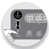
2- The pre-programmed settings can be changed. You can change the time, temperature and speed (refer to the table on the following page) by pressing on the setting that you want to change (C3 or C4 or C5)
