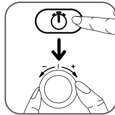
Press **START** key. Set the duration of cooking by turning the selector until the desired time. The digital display tells you the time in hours and minutes (e.g.: 0:45).
