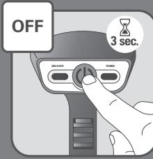
**EN** Press and hold the On/Off button for 3 seconds to switch the appliance off.
