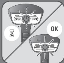
**EN** Plug in and switch on the appliance, then wait until the light stop flashing.
