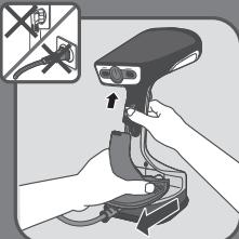
**EN** Unlock and remove the water tank.
