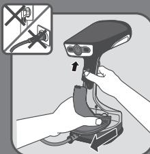
**EN** Unplug the appliance and pull the water tank out.
