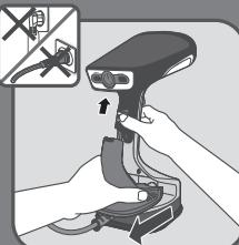
**EN** Unlock and remove the water tank.
