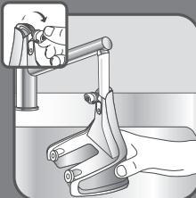
**EN** Remove the water inlet stopper and fill the water tank with untreated tap water.
