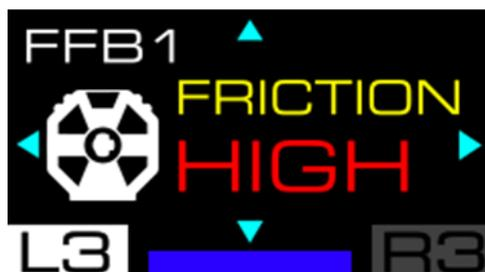
This screen lets you adjust the motor's friction when the wheel rim is turning slowly or not moving. There are four settings to choose from, ranging from no resistance to very strong resistance: OFF; LOW; MID; HIGH.
