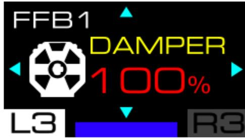
This screen lets you adjust the Force Feedback damper (rotation of the wheel rim that is more smooth or less smooth). This value ranges from 0% to 100%, in increments of 10.
