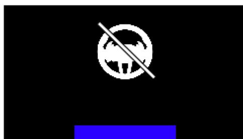
Please install a wheel rim on the base, or uninstall and then reinstall the wheel rim on the base.
