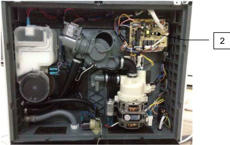
Part name: 1 – protecting box 2 – main control board
