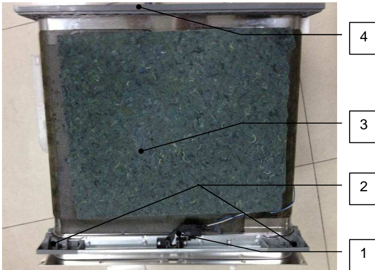
Part Name: 1 – door switch assembly 2 – absorber 3 – 4 –backboard
