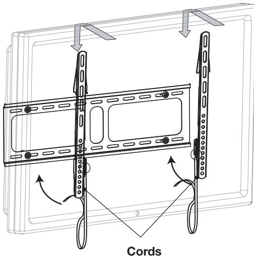
When the TV is correctly positioned, you can fold up the two cords to form a loop.
