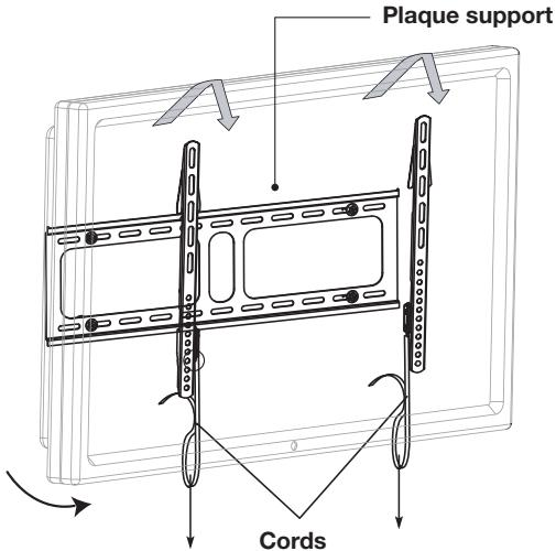
Once the TV is in place, it is possible to remove it from its bracket by simply pulling on the two cords at the end of the mount arms.
