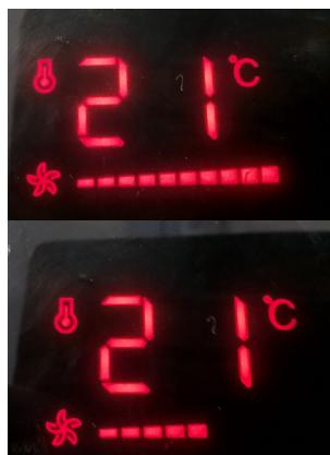
**High intensity:** the appliance runs on full power and the and symbols are displayed on screen. The intensity bar is fully lit. The selected temperature is shown on screen.
