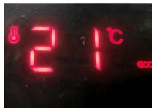
**Eco:** the appliance is running on economical heating power and automatically adjusts the temperature to keep it constant in the room. The
