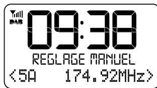
Turn the settings knob to switch between the frequency ranges 5A to 13F.
