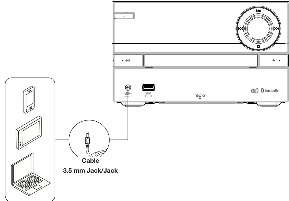
1. Plug the end of a 3.5 mm jack/3.5 mm jack cable (not included) into the socket on the front of the unit.
