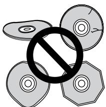
This player is designed to only be used with standard, 100% circular CDs. Do not use CDs in any other shape.
