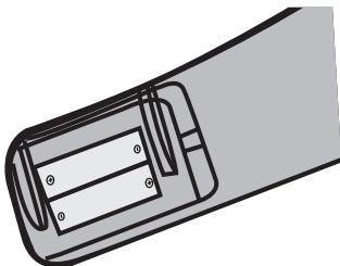
2. Place the batteries in the remote control, respecting the + and - polarities indicated.
