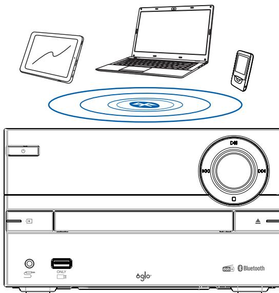
Turn on the micro hi-fi system and select the BT source by repeatedly pressing the
