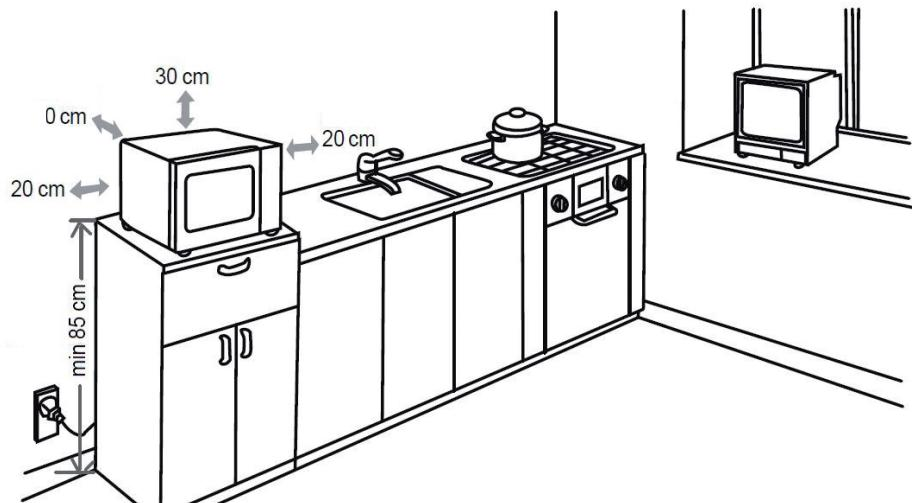
Make sure nothing is blocking the ventilation holes on the sides, top and back of the appliance.
