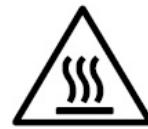
Accessible surfaces (door and exterior surface) may be hot when the appliance is running.
