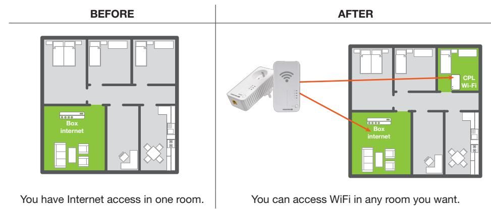
**NOTE:** The Solo WiFi powerline adapter does not allow you to create a network. **At least two powerline adapters** are necessary to create a high-speed network. **The Solo WiFi powerline adapter only allows you to transform an existing wired network into a wireless network.**
