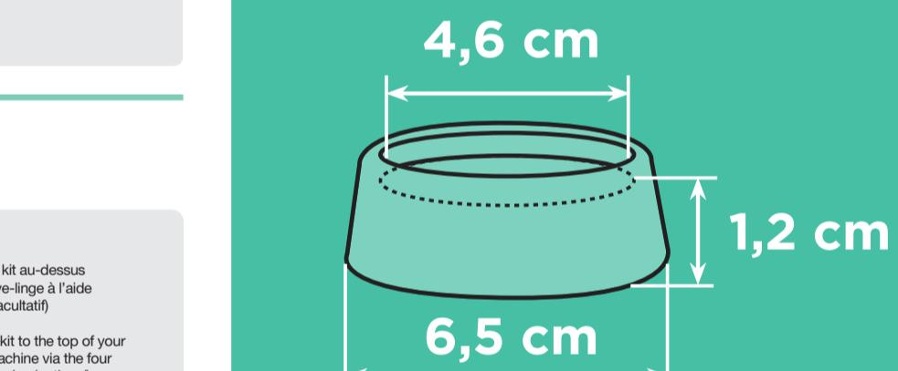
EN Anti-vibration rubber supports for washing machines and dryers (4 pieces). The new, anti-slip rubber formula gives the appliance greater stability.
