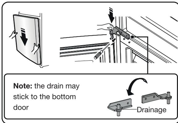
15. Put the top door back on the middle hinge. Pass the electrical wire ③ through the hinge opening ② and then secure the hinge ② with the screws ①.
