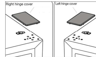
6. Remove the cover (left) ① at the top left of the door and pull out the electrical wire ②. Then, remove the cover (right) ③ and insert the electrical wire ④ into the top right-hand side of the door. Refer to the procedure outlined above. Fit part ③ and part ④ to the top left of the door. Fit part ① to the top left of the door.
