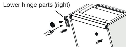
14. Put the lower door on the lower hinge pin and hold it in position. Turn the middle hinge 180°, unscrew and put the washer back under the pin. Adjust the hinge to the correct position and secure it, while making sure the lower door is secure.
