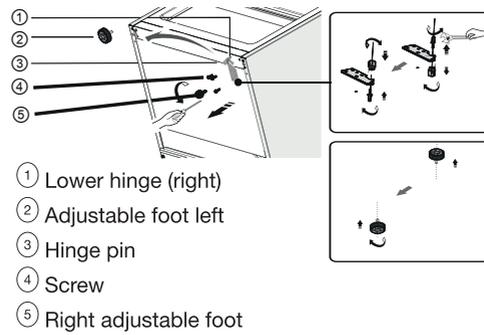
12. Unscrew all the parts of the lower right hinge and remove them.
