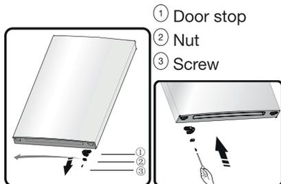
8. Unscrew the screws from the middle hinge and remove the hinge. Then remove the lower door.
