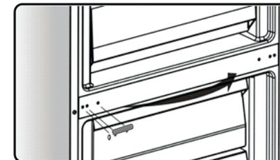
11. Tilt the refrigerator backwards and remove part ②.
