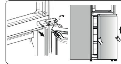
9. Place the door upright on a soft surface. Loosen screw ③ and remove parts ② and ①. Fit the left door stop ④ provided (in the bag of accessories) and part ② (nut) on the left side with screw ③. Store the part ① in the bag of accessories.
