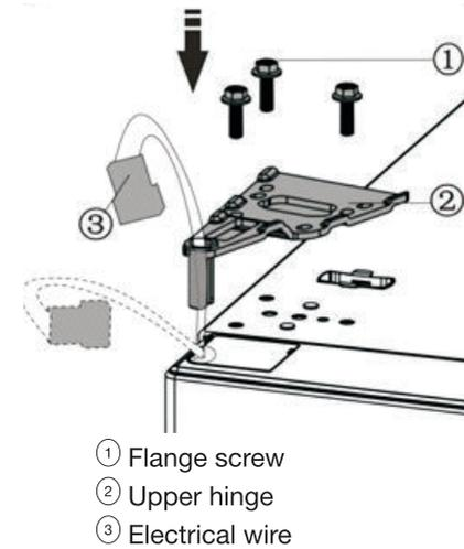
16. Connect the electrical wire ①, as shown below, then secure the top hinge cover ② with the screw ③. Refer to step 2.
