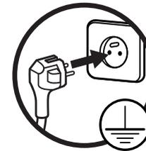
This microwave oven is fitted with an earthed mains plug. It should only be plugged into a correctly installed wall socket with an earth.
