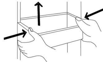
3. As the shelves are equipped with a stop at the back to stabilize them on the appliance, lift them up slightly and then pull them forward as shown in the figure below to remove them before cleaning.
