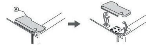
2. Remove the hinge B screw by turning it anticlockwise then remove the hinge. Be careful not to drop the door.
