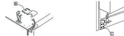
3. Lift the door vertically and remove it from the lower hinge C.
