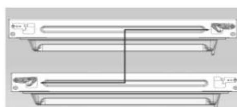
c) Remove the shaft and the two stoppers from the lower hinge and install it in the position, as shown in the following figure.
