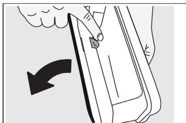
4. Remove the foam filter. Remove lint, fibres and cotton residue by hand or with a soft cloth. Do not clean this filter with water as the filter could become clogged.
