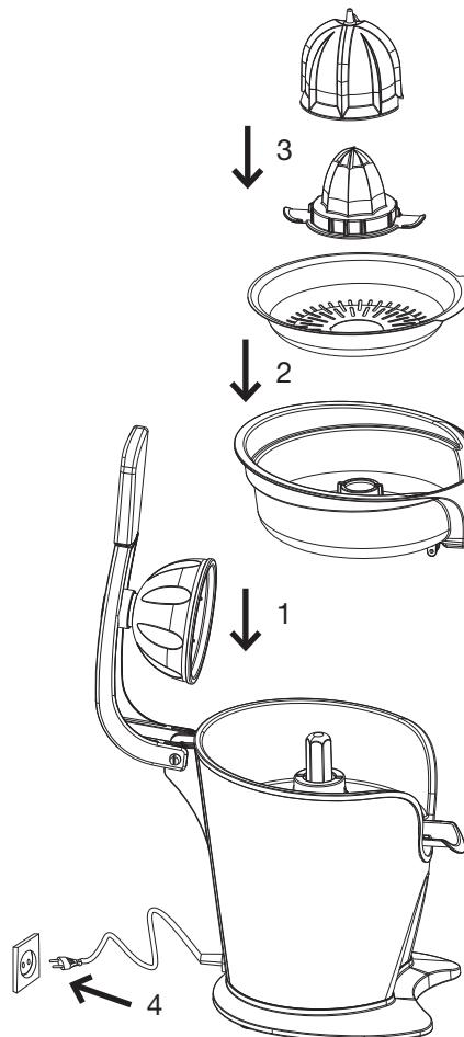
1. Put the juice collector on the motor unit, making sure the pouring lip is either retracted or over a receptacle if it is open.
