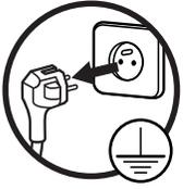
**IMPORTANT:** Unplug the power cord from the socket before cleaning and, if possible, leave the door open to deactivate the microwave oven.
