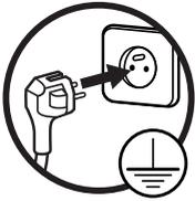
This microwave oven is fitted with an earthed mains plug. In the event of a short circuit, the earth connection reduces the risk of electric shock by providing a route to earth for the current to take.
