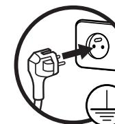
This microwave oven is equipped with an earthed electrical outlet. Earthing reduces the risk of electric shock by allowing a possible short-circuit current to escape through the earth wire.
