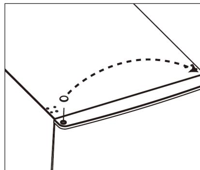
5. Unscrew and remove the bottom hinge pin, turn the bracket over and replace it.
