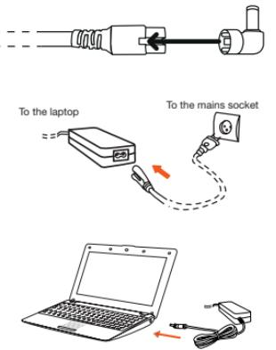
2. Attach the connector to the end of the charging cable, making sure to push it in firmly.
