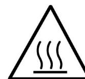
**WARNING:** Do not touch any surfaces bearing the adjacent symbol during or after use when the appliance is cooling down. Danger of burns!
