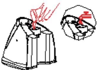
**Warning! Do not overfill beyond the "MAX" level mark.**
