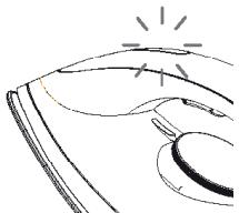
When the iron heats up, the thermostat indicator light is on. The light goes out again when the iron reaches the selected temperature. The indicator light switches on and off during use; it regulates the selected temperature. This is normal.
