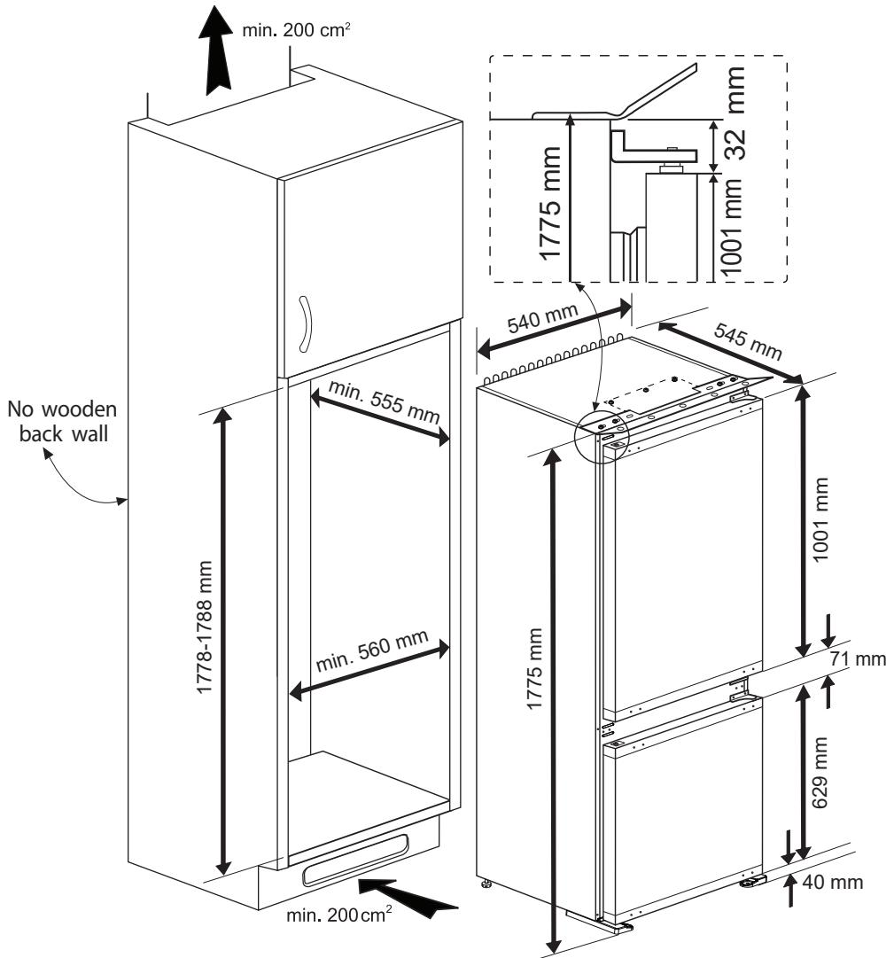
The back wall of the wooden cabinet must be left open completely to the kitchen wall in order to allow sufficient air circulation to cool down the condenser unit for energy efficiency.
