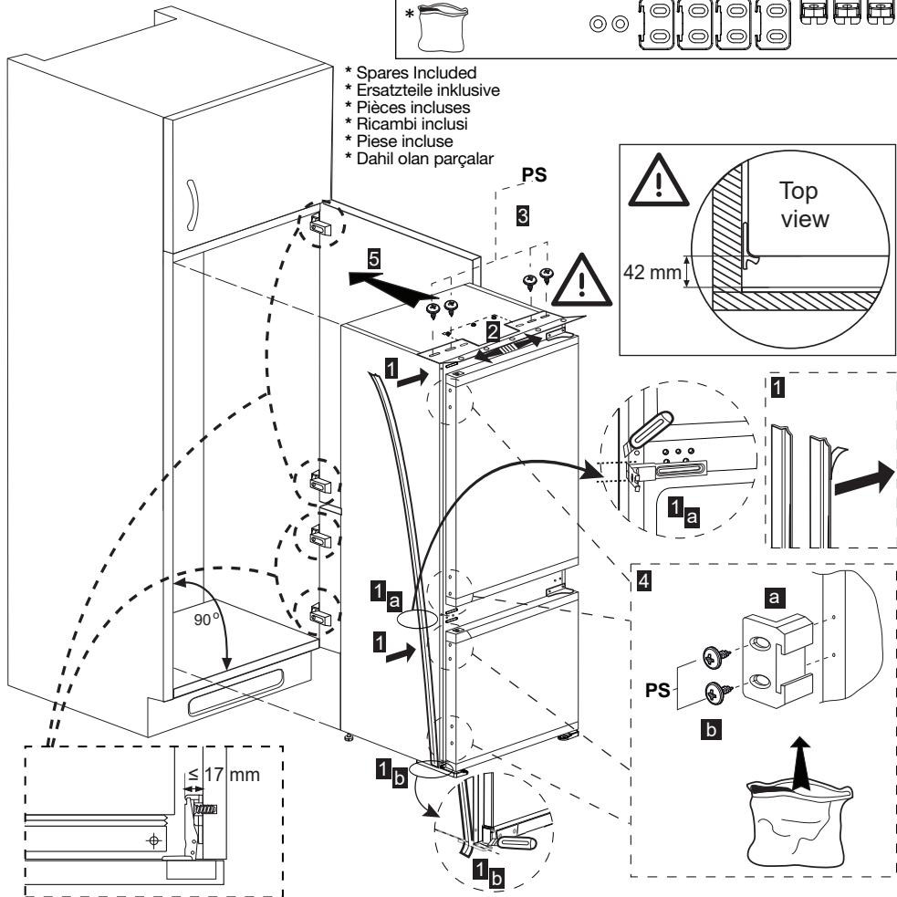
**Note:** Installation step for 2, screws for connecting top plastic part should not be screwed very hard, because of moving the plastic part easily left or right side.
