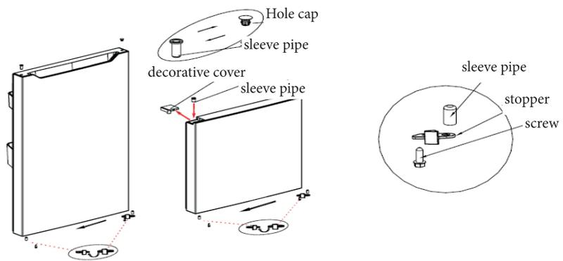
6) Install the Refrigerator compartment door on the lower hinge and then install the middle hinge, screws and caps.
