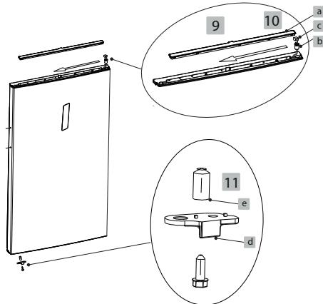
14. Fit the top hinge on the desired side.
