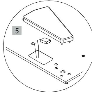
5. On the other side, remove the cover hiding the holes for the hinge.
