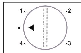
To optimize food preservation, set the thermostat to "2". This setting is appropriate for storing frozen food and maintains the temperature in the freezer at -18°C.
