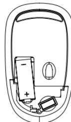
3. Remove the nano-receiver from the compartment. Put the cover back on.
