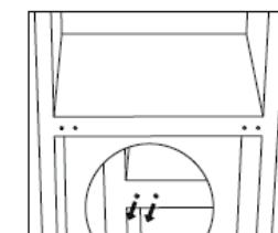
7. Lie the rear of the cabinet on a soft pad. Unscrew the bottom hinge and levelling foot.
