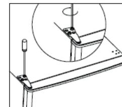
14. Clip in the hinge cover and hole cover on the top of the unit
