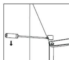
4. Move the core cover from the left side to the right. Then lift the upper door and place it on a padded surface to prevent it from getting scratched.
