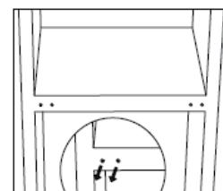
11. Stand the unit up and put the door on the bottom hinge. Make sure the bottom hinge core is inserted in the door hole. Then move the hinge hole cover of the bottom door from the left side to the right.
