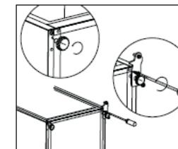
8. Unscrew and remove the bottom hinge pin, turn the bracket over and replace it.
