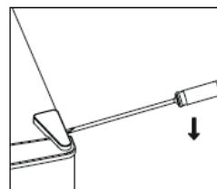
2. Unscrew the top hinge with a cross-headed screwdriver.
