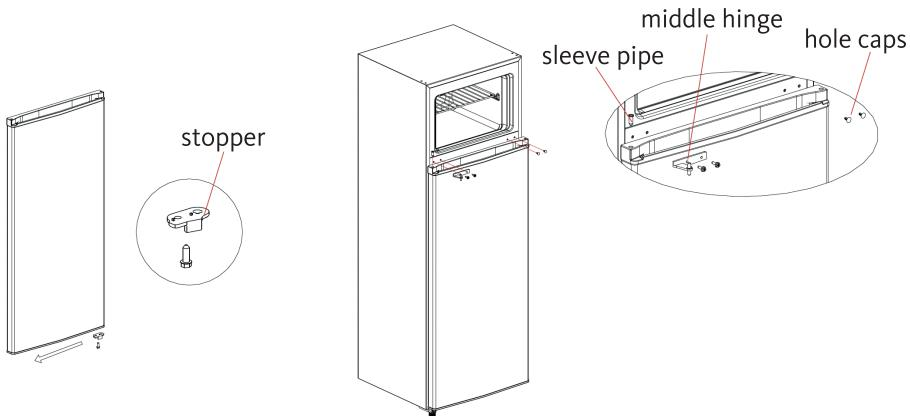
8. Assemble the stopper of the freezer door on the other side.
