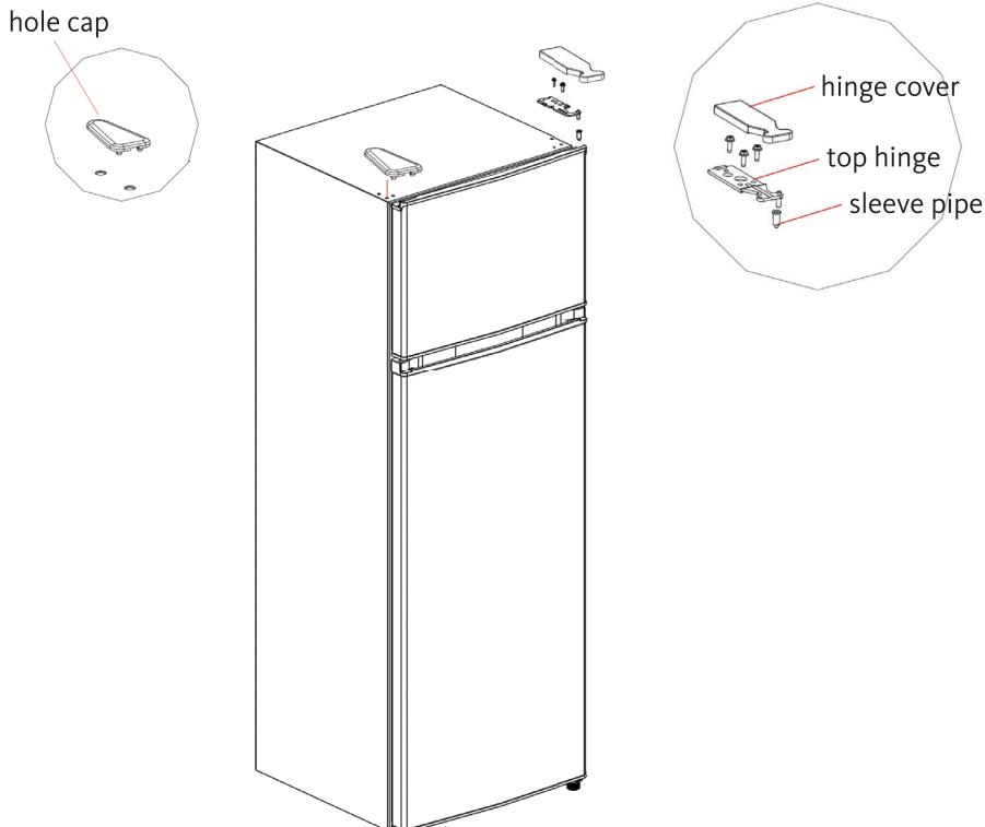
3. Take off freezer chamber door, middle hinge, the sleeve pipe of refrigerating door and hole caps on the other side.
