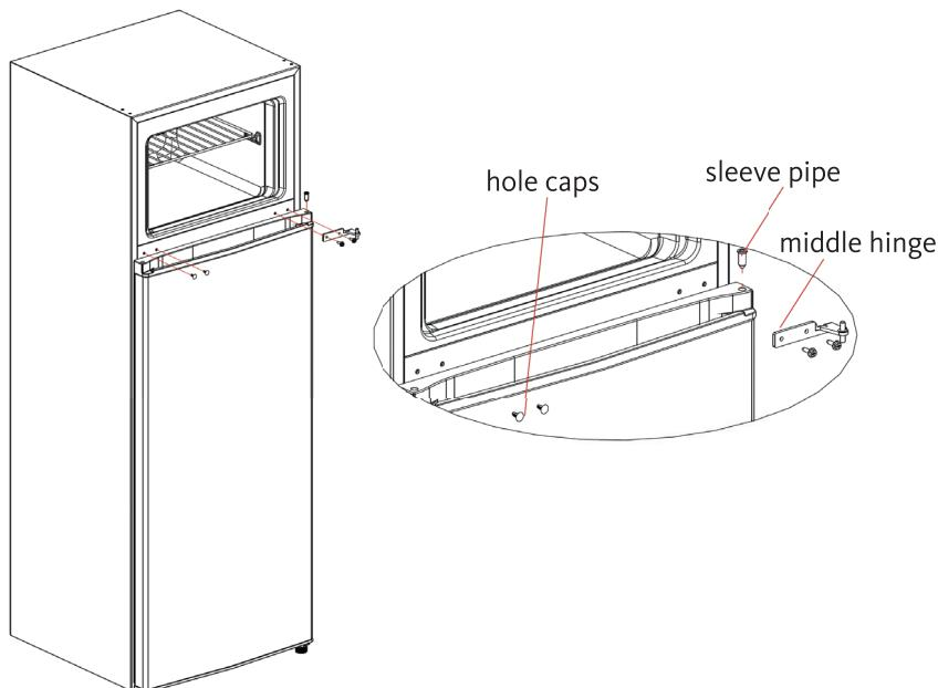
4. Remove the refrigerating door, remove the bottom hinge and adjustable foot on the other side.
