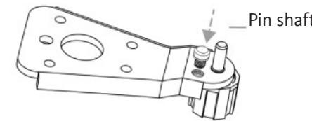
9. Install the lower hinge on the left side of the cabinet.
