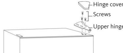
3. Remove the refrigerator compartment door from the cabinet.
