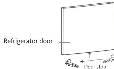
16. Install the Refrigerator compartment door.
