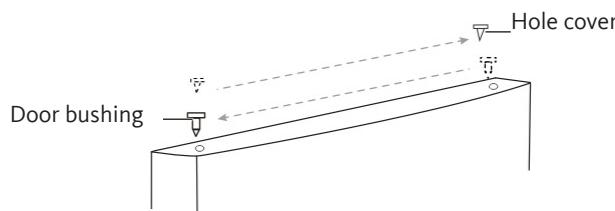
18. Remove the hole cover from the top left side of the cabinet and secures the cover on the top right side of the cabinet.
