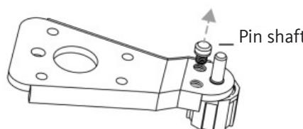
8. Insert the pin shaft into the left hole on the lower hinge, then secure the shaft with the washer and nut.
