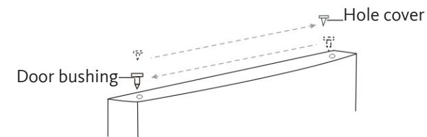
13. Remove the center hinge screw hole plug on the left side of the cabinet, then install in the screw holes on the right side of the cabinet.
