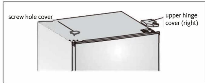
3. Unscrew the special flange self-tapping screws which are used for fixing the right upper hinge part by a 8mm socket driver or a spanner (please support the upper door with your hand when doing it).
