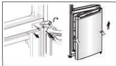
8. Place the lower door on a smooth surface with its panel upwards. Loose screw ② and part ①, then install them to the left side and tighten securely.
