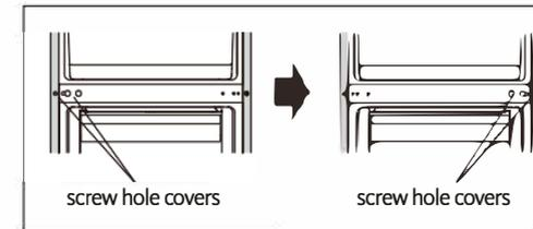
10. Lay the refrigerator on soft foam packaging or similar material. Remove both adjustable bottom feet parts, and remove the front feet board and the lower hinge part by unscrewing the special flange self-tapping screws.
