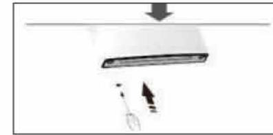
9. Change screw hole covers on middle cover plate from left to right (as shown in figure below).
