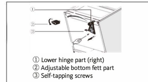
11. Replace the lower hinge part to the left side and fix it with the special flange self-tapping screws. Replace the adjustable bottom feet parts to another side and fix it.
