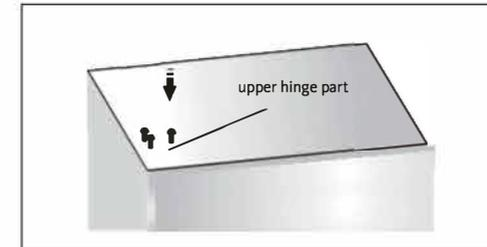
16. Install the screw hole cover on the top right corner of the refrigerator. Install the upper hinge cover (which is in the plastic bag) on the left corner. Put the other upper hinge cover into the plastic bag.
