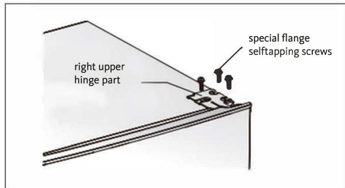
4. Remove the upper hinge axis, transfer it to reversed side and tighten securely, then put it in a safe place.
