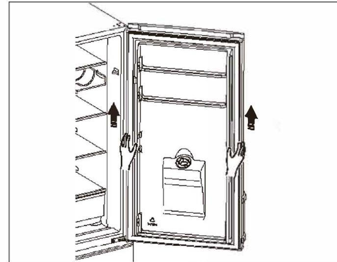
6. Place the upper door on a smooth surface with its panel upwards. Loose screw ② and part ①, then Install them to the left side and tighten.
