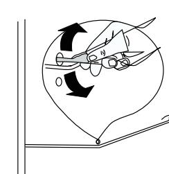
This drainage mechanism can get dirty very easily and cause unpleasant odours; make a habit of cleaning it regularly.
