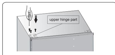
16. Install the screw hole cover on the top right corner of the refrigerator. Install the upper hinge cover (which is in the plastic bag) on the left corner. Put the other upper hinge cover into the plastic bag.
