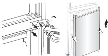
8. Place the lower door on a smooth surface with its panel upwards. Loose screw ② and part ①, then Install them to the left side and tighten securely.
