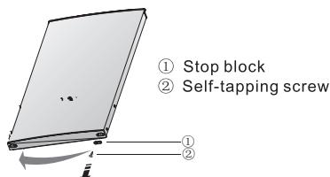
7. Unscrew the two special flange self-tapping screws which are used for fixing the middle hinge part, then remove the middle hinge part that hold the lower door in place.
