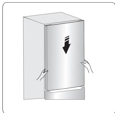
15. Transfer the upper hinge part and make the upper hinge axis into the upper hole of the upper door, and adjust the position of the upper door (please support the upper door with your hand when doing it), fixing the upper hinge part with the special flange self-tapping screws.
