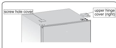
3. Unscrew the special flange self-tapping screws which are used for fixing the right upper hinge part by a 8mm socket wrench or a spanner (please support the upper door with your hand when doing it).
