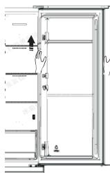
6. Place the upper door on a smooth surface with its panel upwards. Loose screw ② and part ①, then Install them to the left side and tighten securely.
