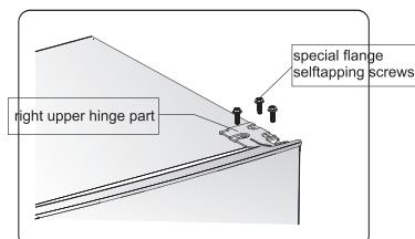
4. Remove the upper hinge axis, transfer it to reversed side and tighten securely, then put it in a safe place.
