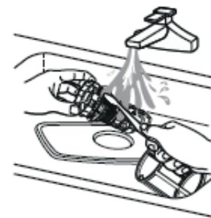
5. Reassemble the filters in the reverse order of disassembly, replace the filter group and turn it clockwise to the arrow corresponding to the closed position.
