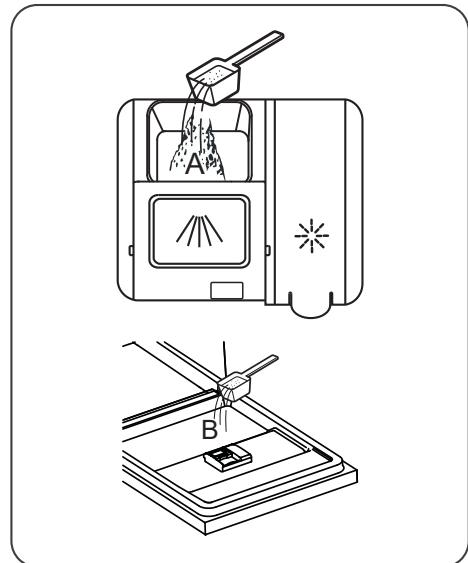
2. Add detergent to the larger recess (A) for the main wash cycle. For best results, especially if the dishes are very dirty, pour a small amount of detergent into the small recess (B). This additional detergent will be used during the prewash phase.
