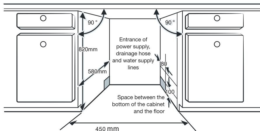
2. If the dishwasher is installed next to a corner cabinet, leave sufficient space to open the door.
