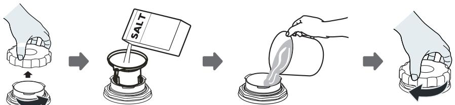
1. Pull out the bottom dish rack and unscrew the cap on the salt compartment.
