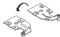
12. Remove the screw hole cover ①, then install it to the right side ② , as shown in figure below.
