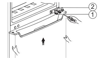
5. Place the lower door on a smooth surface with its panel upwards. Loose screws ①, and remove part ②, then install part ② to the left side with screws ①.
