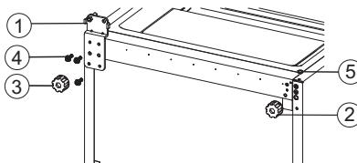
10. Move the lower door and adjust its position to align lower hole site and upper hinge axis. Turn the middle hinge by 180, adjust the middle hinge to the appropriate position and then install it.
