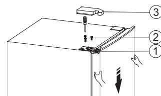
Note: When installing part ③, firstly, push it from left to right completely, then push it down tight.
