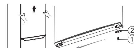
4. Loose screws ① used to fix the middle hinge ② and remove middle hinge ②. Then remove the lower door.
