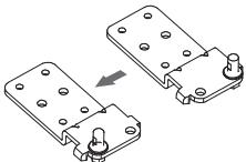
9. Just remount to the step 7, change part ① to left and part ②, ⑤ to right and then fix part ① with screws ④. Finally install part ③ .
