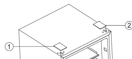
13. Move the upper door to appropriate position, adjust part ① and upper door, and then fix part ① by screws ② (Please hold upper door by hand when installing) , and then install another part ③ (in the plastic bag).
