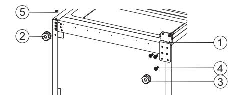
8. Screw out lower hinge, change it to the near hole site, and then screw up.
