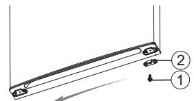
6. Change screw hole covers on middle cover plate from left to right (as shown in figure below).
