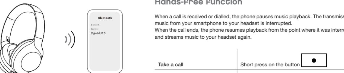
The headset is equipped with multipoint technology. This allows you to pair a second Bluetooth® device with your headset and to choose to take a call from either device.
